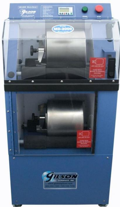
Gilson offers the ideal equipment for micro-deval testing of aggregate materials. Their MD-2000 micro-deval apparatus (<https://www.globalgilson.com/micro-deval-apparatus>) showcases simple, practical feature with several unique considerations.
